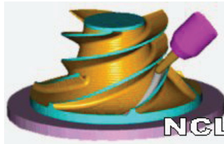
5 axis milling, full contouring
